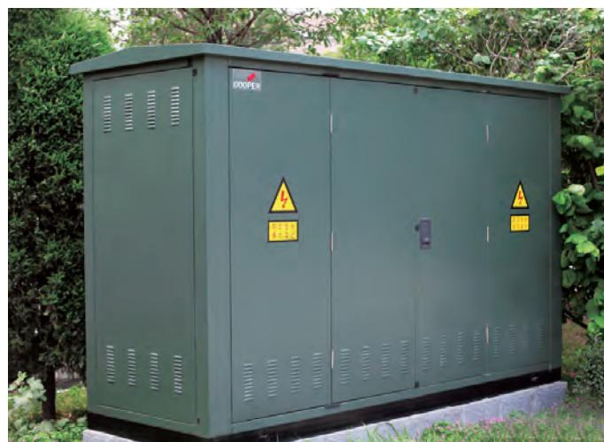
Based on the design concept of full insulation and fully sealed, all primary parts within RVAC RMU are fully sealed inside the stainless-steel main enclosure, protect against condensation and external contaminated environment; the protection degree of the main tank body is up to IP67, equipped with Cooper's water-proofing touchable cable bond, which can provide effective protection against accidental flood in rainy climate.
